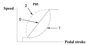
User can customize the speed adjustment performance of the pedal. To start up quickly, select P05=2; to start up smoothly, select P05=1.
