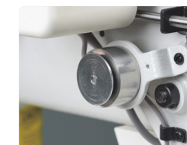
电子松线，起缝更稳 Electronic thread loosening for stable stitch start
